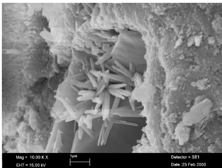
Fig. 3. SEM picture of a cement containing 1% (w/w) of silicone in the solid phase.
